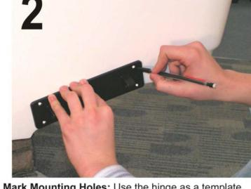
Mark Mounting Holes: Use the hinge as a template. Also make sure that you can mount the hinge in the same location on the other side of the boat.
