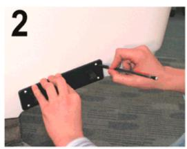
Mark Mounting Holes: Use the hinge as a template. Also make sure that you can mount the hinge in the same location on the other side of the boat.
