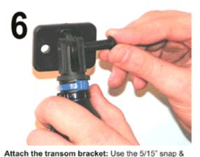
lock pin to attach the transom bracket to the TOP of the Actuator (two cable clamps).
