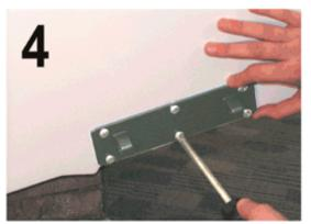
Install the hinge: Use small amount of marine sealant in each hole. Do not use excessive force when installing screws - ream the hole if necessary.
