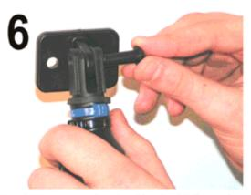
Attach the transom bracket: Use the 5/15" snap & lock pin to attach the transom bracket to the TOP of the Actuator (two cable clamps).
