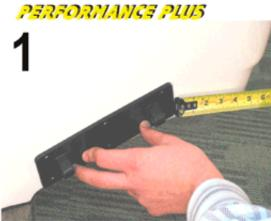
Choose The Location: Preferably 3" to 5" from the outside edge of the transom. Align the bottom of the hinge flush with the bottom of the transom.
