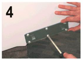
Install the hinge: Use small amount of marine sealant in each hole. Do not use excessive force when installing screws - ream the hole if necessary.
