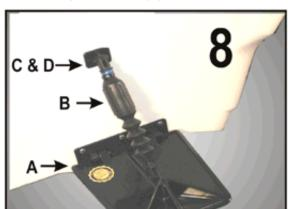
Attach the Actuator: Use the 5/16" snap & lock pins to attach the bottom of the actuator to the trim plate in Hole #3. NOTE: If needed, pressure adjustments can be made to suit your boat after a sea trial.
