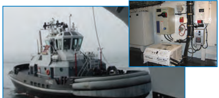
Military tugs utilize inverters as AC UPS as back-up to on-board generators.
