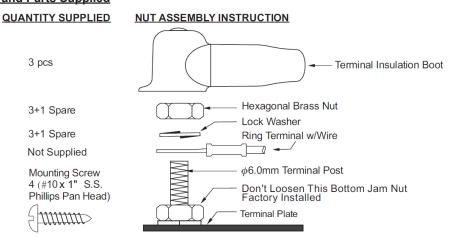
NOTE: Install hardware to the studs in the order as shown above.
