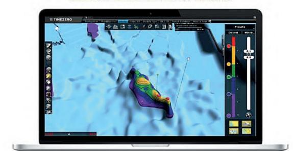
When connected to a sounder which has a bottom discrimination feature, the PBG Module allows TIMEZERO to register the seabed information in addition to the depth. TIMEZERO can then display Bottom Classification as well as bottom hardness using a color scale on the chart.
