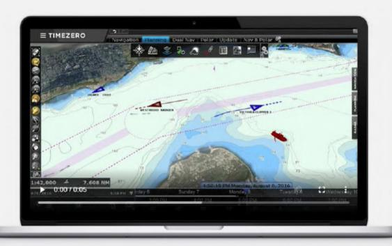
VDR offers the possibility to save all the information received from the connected sensors to TZ Professional (GPS, Radar, AIS, etc.) It is particularly useful in the case of an incident as it allows one to look back at all the available information relative to the surrounding environment of the boat at that given date and time.
