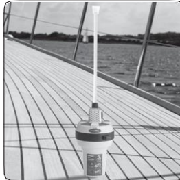
b) EPIRB deployed on deck
