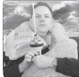
c) EPIRB used in a liferaft.
