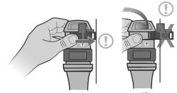
Pass the loop at the end of the Activation Tape through the slot in the Activation Slide and pass the tape back through the loop. Return the Activation Slide to the centre and move the red Arming Slide back to lock the slide in place.
