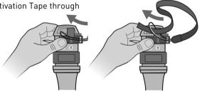
Take the lifejacket Fixing Buckle (Supplied) and pass the tape through the slots as shown below, making sure that tape does not get twisted.
