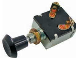
#5521PT (#5521C) On-Off Push-Pull SPST Pull For On 2 Screw Terminals 1/2" Mount Hole 6 Volt 25 Amp 12 Volt 15 Amp
