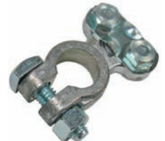
Universal Emergency Lead Terminal Fits Most Batteries #0880 Fits 6 - 1 Ga #0888 Fits 1 - 4/0 Ga
