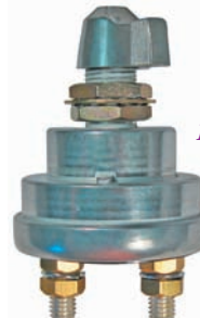
#5574PT (#5574C) Master Battery Disconnect 2 Stud Terminal 3/4" Mount Hole For Battery Circuit Only On - Off SPST 6-36 Volt 190 Amp DC Continual 1000 Amp DC Momentary
