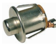
#5508PT (#5508C) Universal Starter Switch With Ground Receptacle Push Button Momentary On Snaps Into 15/16" Hole 6 Volt 15 Amp 12 Volt 10A / 24 Volt 6A
