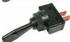
Black Toggle Black Nylon Housing 1/4" Male Tabs / 1" Handle Length 1/2" Mount Hole 12 Volt 16 Amp
