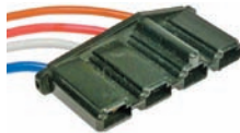
#5438PT (#5438C) Voltage Regulator Repair Harness 4-18 ga Leads GM 1961-73 Delco 7700 GM 88860584 PT2029
