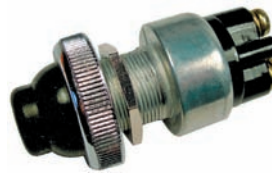
#5509PT (#5509C) Heavy Duty Push Button Momentary On Rubber Dust & Moisture Resistant Boot Nut 5/8" Mount Hole 12 Volt 60 Amp
