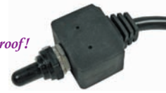
#5589PT (#5589C) Momentary On-Off- Momentary On Toggle SPDT - 3 Position Waterproof Bat Handle With Boot 3 6" 16Ga Jacketed Wire Leads 1/2" Mount Hole 12 Volt 25 Amp
