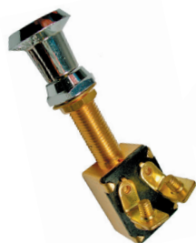
#5528PT (#5528C) Push-Pull Brass Switch On-Off SPST Chrome Plated Knob 2 Screw Terminals 3/8" Mount Hole 6 Volt 25 Amp 12 Volt 15 Amp
