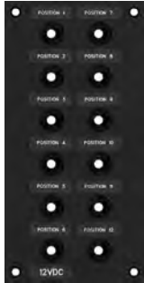
7226 4.50" W x 9.00" H x 2.50" D DC 12 Position Push-to-Reset Circuit Breaker Panel 9997226 Black, 12/24 VDC, Loaded with 12 - 15Amp Push-to-Reset Circuit Breakers
