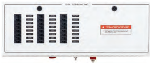
Main DC Control Engine Room Panel with enclosure protection. Includes: ignition protected circuit breakers, solenoids, relays, ANL fuses, wire access ports, external connectors and power studs. Key locked access for easier and safer service.
