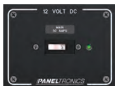
1202 5.5" W x 4.125" H x 3.5" D DC High AMP Breaker Panel 50A Standard (60, 80, and 100A available)
