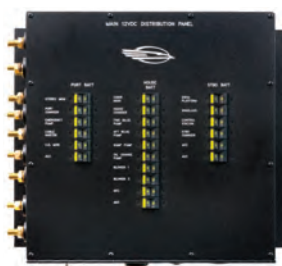
Ignition Protected Main DC power distribution enclosure assembly. Includes: battery switching solenoids, circuit breakers, fuse blocks, relays, external power studs and connectors.
