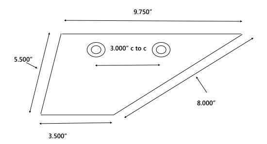
Made of 316 Marine Grade Stainless Steel Thickness: 1.5 mm
