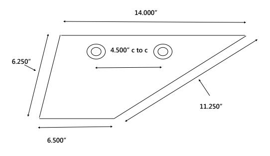
Made of 316 Marine Grade Stainless Steel Thickness: 1.5 mm
