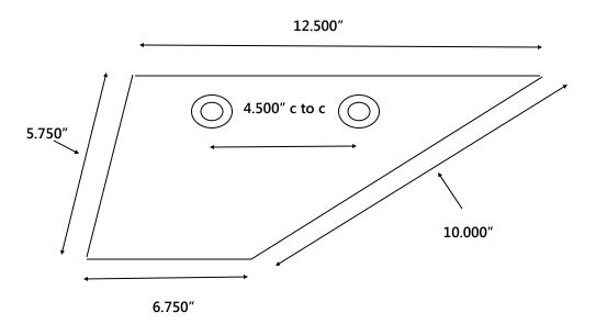
Made of 316 Marine Grade Stainless Steel Thickness: 1.5 mm .625"
