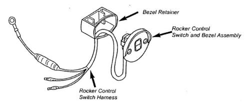
**NOTE**: The bezel retainer is mounted onto the switch bezel before placement into opening. A gap between the bezel and the bezel retainer must be 1/8" (3.2 mm) greater than the thickness of the mounting surface.
