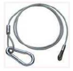
When using the motor lift on open water, attach the included **Outdoor Motor Safety Cable** (see picture on left—part #55-0415) to the boat and motor lift. This is a vinyl coated 3/32" diameter, 50" long heavy duty steel cable with one loop and one snap hook.
