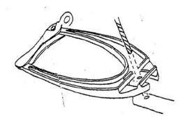
By removal of wing nut "Happy Hooker" can be turned over to be refitted at right angles to pole to facilitate the engagement of a ring with a limited clearance behind it.
