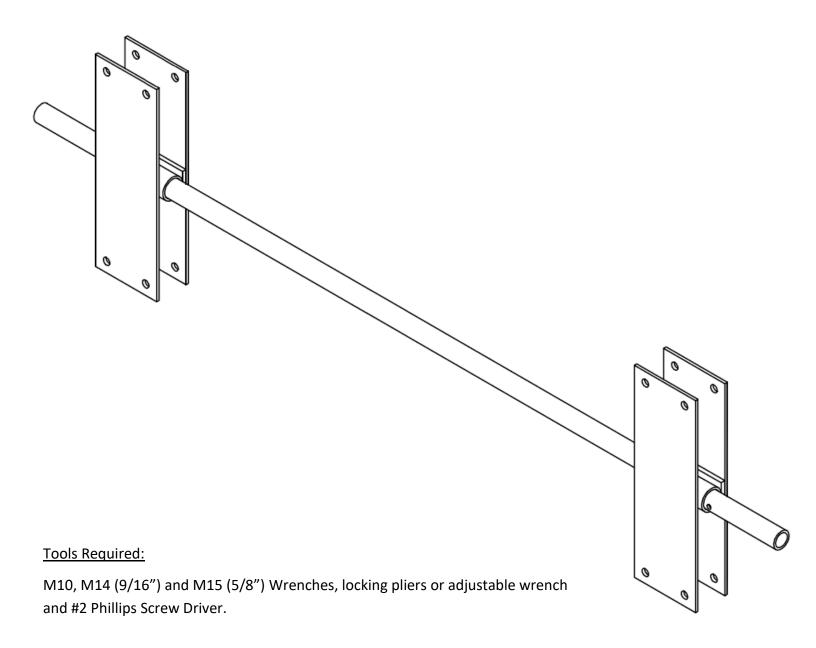
\*NOTE\* Each Patriot frame being joined together by the hinge must have a PN10803 End Rail installed on each side of the joint.
