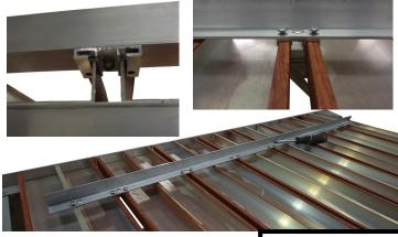
To assemble the <u>aluminum deck panel</u>, lay out the deck boards, slide stinger onto boards. Position stringer approx. 12" from edge. Repeat with other stringer on opposite side. Ensure board ends are flush. Tighten set screws to secure panel.
