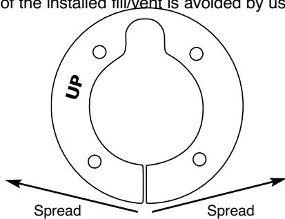
2. Unfasten the fill/vent from the mounting surface, then pull it up a half inch, spread the ring approximately 2 inches apart at the split, and slide the ring under the flange, keeping the "UP" side facing the flange. Black RTV type silicone sealant may be applied to the top, bottom and split surfaces of the ring, if necessary.
