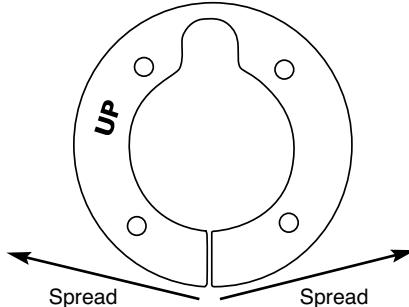
2. Unfasten the fill/vent from the mounting surface, then pull it up a half inch, spread the ring approximately 2 inches apart at the split, and slide the ring under the flange, keeping the "UP" side facing the flange. Black RTV type silicone sealant may be applied to the top, bottom and split surfaces of the ring, if necessary.
