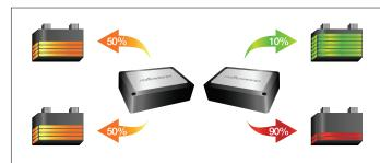
The Adaptive Loading feature dynamically adjusts the charger's output level on each output bank. More charging power is allocated to battery that is low in charge, and less charging power to battery that is closer to being fully charged.
