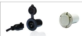
The Powermania AC Plug Port is designed to work with only Powermania charger's AC plug. It provides a thru-hull AC connection between the charger and AC extension cord. The installation does not require any cutting or stripping of the AC cord. The AC Plug Port's cover seals the AC plug from water and corrosion when it is not in use. The AC Plug Port is available in black and white.
