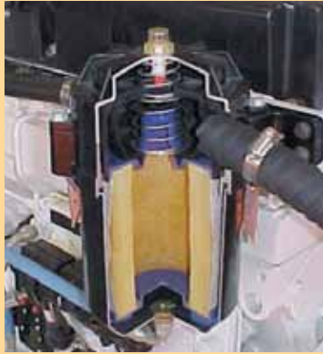
Cummins QSM11 marine engine with CCV cutaway
