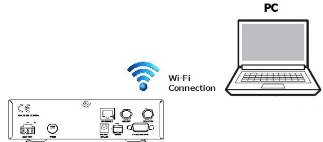
Figure 23 : ACU to PC Wifi Connection
