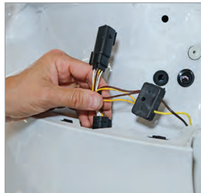
3. Route T-Connector to the tail light harness.
