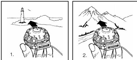
The Ritchie SportAbout™ is a Direct Reading Compass. The Bearing you read on the dial is the direction you are facing.
