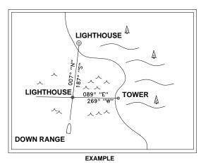
**Step Four.** Check compass alignment by running the boat in a Southerly direction, again keeping the marks lined up. If the compass is not correct at this time, there is an alignment error. To correct, rotate the compass itself to remove one half of this error. Repeat steps 1, 2 & 4 until your North/South line is correct then repeat step 3. **Step Five.** Install fastener (s), taking care not to disturb alignment.
