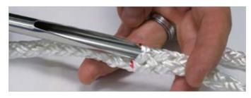
At mark 2, stick the splicing needle into the core and move it toward mark 3.
