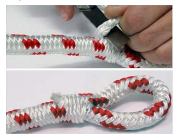
Pull the core toward the eye and cut it off very close to the exit point. Be sure to avoid damaging the cover when cutting off the core.
