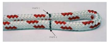
Define the desired eye size and mark the rope again in the appropriate location (mark 2)..
