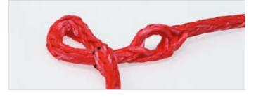
Open the tipped rope end after 2 plaits (2 - 3 cm) again in the center (equal number of strands on both sides). This is the second opening.
