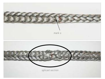
Once the splicing procedure has been completed, no rope end should be projecting at mark 2, on either side.
