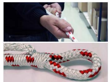
Attach the knot from step 9 to a securely anchored hook and slip the cover gradually toward the eye of the splice.
