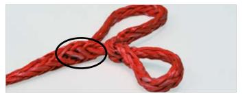
Insert the tipped end into the rope. After 30 cm, guide the tipped end out of the rope again (see the following photo).
