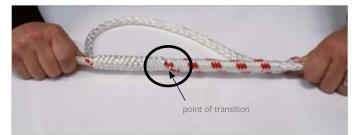
Using both hands, pull at the taped up ends (core and cover). Make sure that the point of transition is pulled together tightly.
