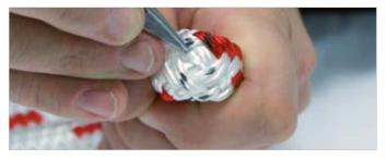
Bend the rope sharply at mark 2. Using an awl, open the rope's cover.
