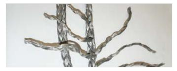
Then, the rope ends pulled outwards need to be tapered symmetrically by 50%. (In the case of a 12-strand braiding, only six strands will remain on the last approx. 25 cm)
