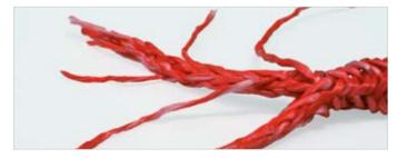
Remove the adhesive tape and taper the rope's end such that 30% to 50% of the strands are extracted from the rope's end at equal distances and severed.
