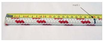
Mark the rope in a location 20 cm from the end of the rope (= mark 1)
