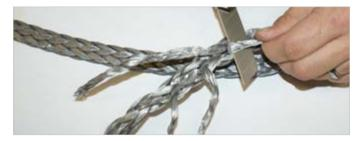
Cut off the projecting ends close to the rope.
