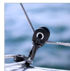
Cheek plates twist to open block
