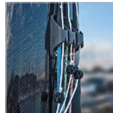
Release lanyard in 'open' position
