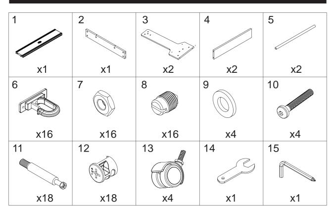
Attention: If you are using an electric screwdriver in the assembly, please set at low torque and do not over tighten the hardware. When assembling individual parts, loosely tighten screws until all screws are inserted, then tighten completely.
