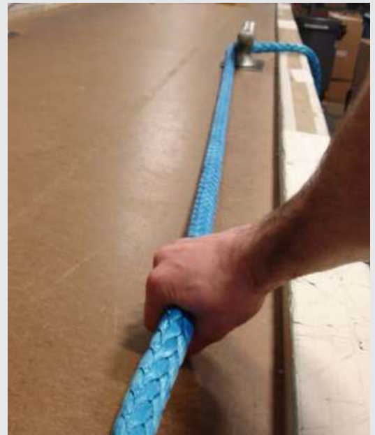
Tension rope with hand force and measure to reduce the variability in length.
