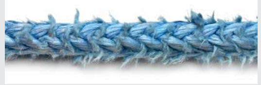
Abrasion occurs both externally, along the surface of the rope and internally, inside the structure of the rope. It is important to evaluate both forms to accurately assess the condition of the rope.
