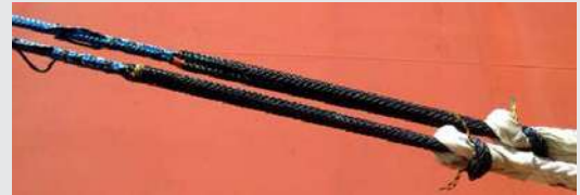
Using a braided pendant with a braided mainline will reduce the likelihood of twisting the mainline.
