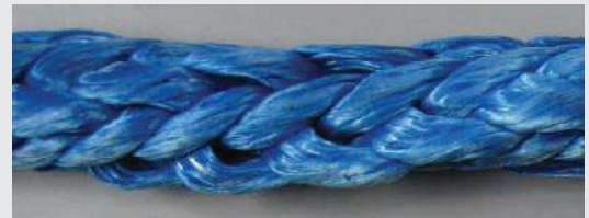
FIGURE 1 The loose strands at the top of the rope do not contribute to the strength of the rope. The tight strands at the bottom of the picture bear most of the load.
