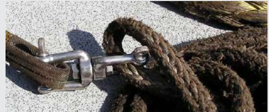
Using a swivel to connect the messenger line to the mainline or pendant can reduce twist in the pendant and mainline.
