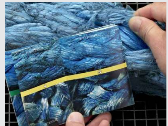
The comparator is an easy reference that can be used in the field to help assess the state of a rope. Small and easily held in the hand while performing an inspection, it helps establish a guideline and a common language when discussing the state of a rope.
