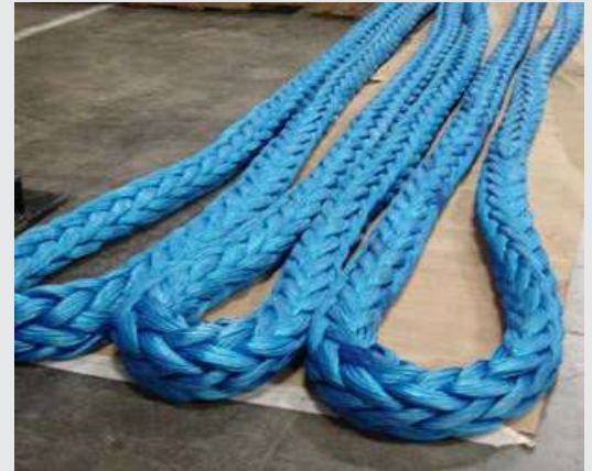
Do not allow the length of rope being measured to be curved or twisted.
