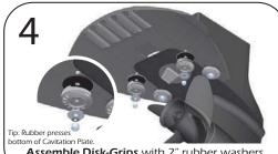
Assemble Disk-Grips with 2" rubber washers, 1" & 5/8" washers and nuts hand tightened.
