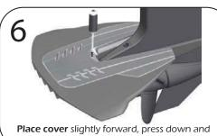
slide back to hold in place, & install screw.
