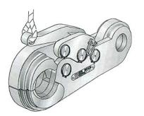
**Sea Catch TR15LM** This is a modified TR15 provided with a front jaw enlarged to receive up to 3.4" fibre line. Additional side plates at the jaw area help spread the load and prevent line chafing. Other capacities are available.
