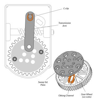
b. Remove the C-clip from the end of the transmission arm using a flat blade screwdriver and lift off the Transmission Arm by pressing down lightly on the gear wheel to release.
