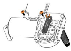
a. Using a Phillips head screw driver, remove the four screws from the shaft plate and carefully remove the shaft plate and red gasket.
