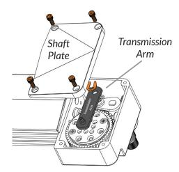
a. Using the provided Allen wrench, remove the four screws from the shaft plate and carefully remove the shaft plate.
