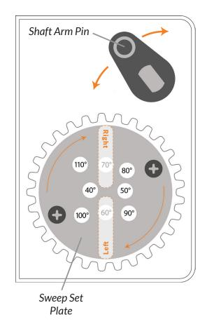
a. Using a Phillips head screwdriver, remove the two screws holding the sweep set plate to the gear wheel and then rotate the Sweep Set Plate a full 180°, reloacating the desired sweep set hole over the oblong slot on the opposite side of the wheel.
