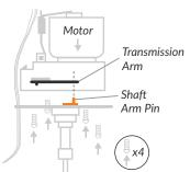
a. Making sure the shaft arm pin is placed into the hole at the opposite end of the transmission arm, replace shaft plate to the inner motor and attach with the four inner screws.
