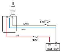
All Sea-Dog wiper motors have the "coast-to-park" features, which means that when power is cut to the motor, the motor will "coast" to its original set position at the bottom or top of the windshield.
