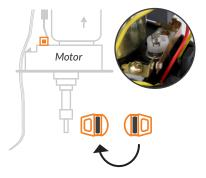
Using a small flat tip screwdriver, remove the plastic cam, rotate it 180°, and replace.
