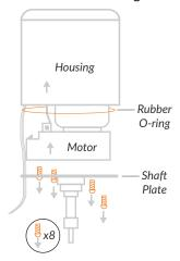
Remove eight screws from the shaft plate and carefully remove the shaft plate and inner motor from housing. (note the placement of the small black o-ring in the channel of the housing) 2. Adjust Transmission Arm
