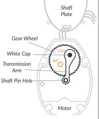
Inside the motor, remove the white cap holding the transmission arm in place then relocate the transmission arm to the desired sweep set:
