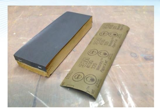
The wet sanding process begins with 320g paper. An easy D.I.Y. system uses a standard sheet of sandpaper cut to fit a 9.5" sanding block and stapled in place. The 320g finish can be followed by 400g, 600g or even finer depending the finish desired.
