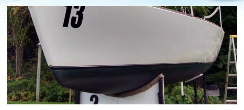
This is the same Biocop TF racing finish after 2 seasons in New England. Notice the color difference several inches down from the waterline. All Cukote and Biocop TF colors will change slightly with the burnishing process.
