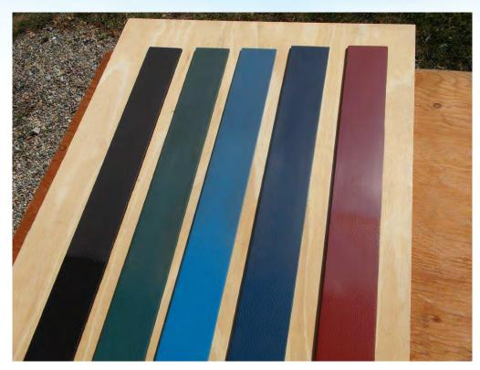
The top half of each of these panels has been wet sanded to a 600 grit finish. The bottom half of the panel is just as it was rolled. 4 coats were applied.
