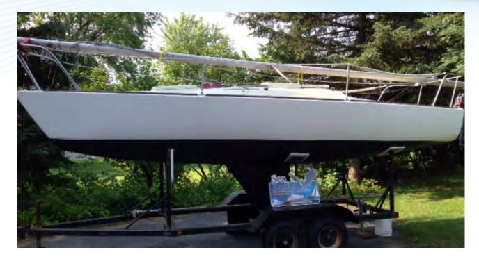
This is a freshly sprayed Biocop TF black bottom. About 50% more paint was applied than normal in anticipation of a wet sanded racing finish. Allow the paint to cure for about a week prior to burnishing the finish.
