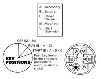
**NOTE:** These switches are intended for manual operation only and are not intended for use in conjunction with emergency ignition shut-off devices which are attached to the control box or switch housing to mechanically rotate the switch key to the "OFF" position.
