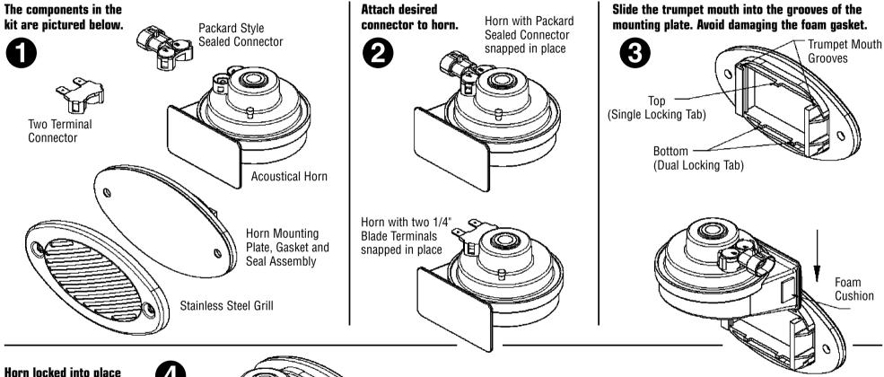
Horn locked into place between top and bottom locking tabs.
