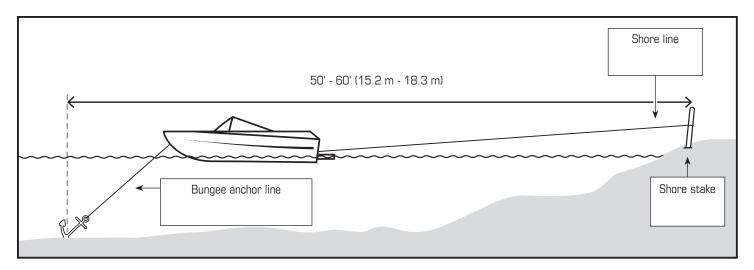
3. Release portion of shore line and allow vessel to be pulled back to deeper water. Make sure the shore line is still secured to the stake.
