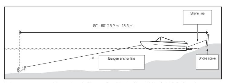
2. Secure rope to stern and shore stake and pull boat to shore. Tie off and board/deboard, load/unload vessel.
