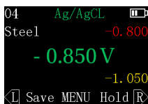
Figure 6 Corrosion Measuring Screen
