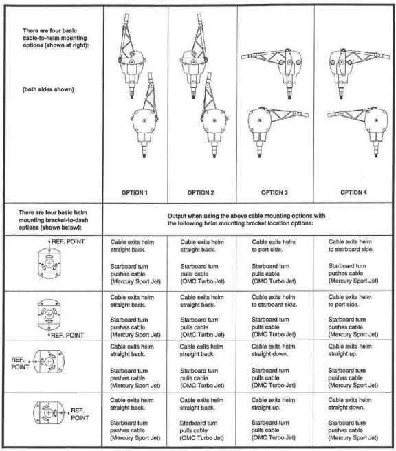
NOTE: In addition to the above mounting bracket options, slotted mounting brackets allow 20° of helm rotation in both directions.
