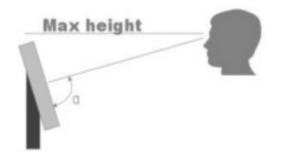
Viewing angle is an theretical value measured with standard colors and contrast. In real life the monitor should be installed with angle: 120  $< \alpha < 90$ . This means that viewing from bottom side should be avoided. For viewing convenience install the monitor below eyelevel (max height).
