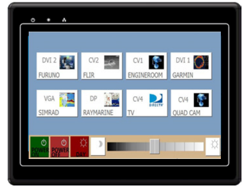
Monitor Screen - Press buttons to change screen input signal. Press and hold a button to set it up.
