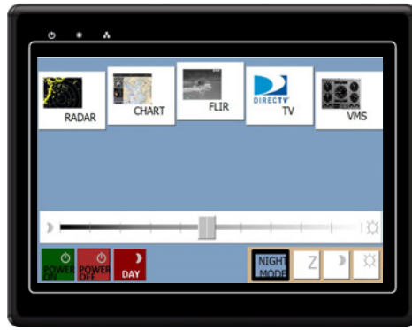
Monitors - Select a monitor to change its display. Use Preset buttons on bottom to display predefined configuration.
