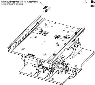
4. Slide the Square Linear Bearing (SW-0549I) onto the starboard square rail from the rear of the module.
