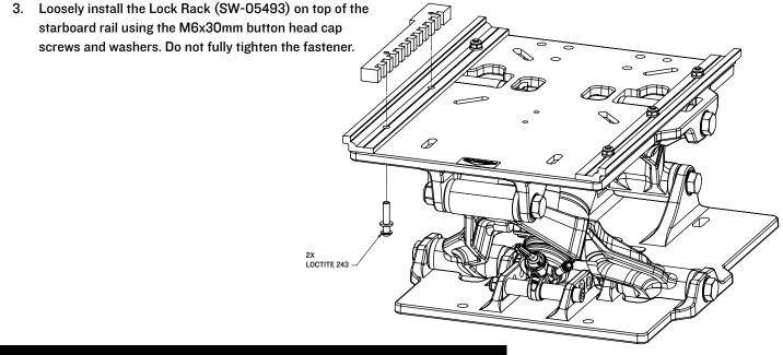
**IMPORTANT** If your module is equipped with height adjust, use M6x25mm button head cap screws and washers.
