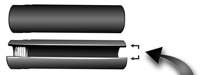
The highlighted area above should be cut away using a band saw. If this is not available, contact your local machine shop to perform the task. The section, when removed, should be between .3150 inch to .3250 inch wide.
