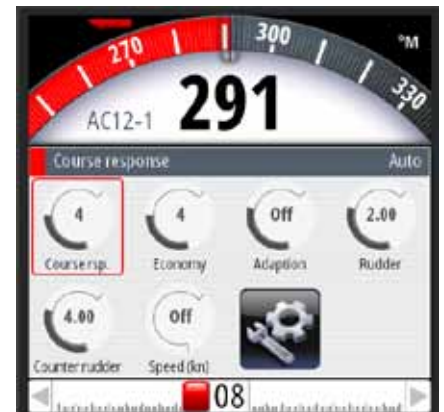
Steering parameters are clearly viewed and easily adjusted.
