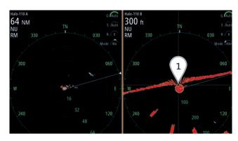
▲ **300FT AND UP TO 72NM - SAME TIME & SCREEN** Halo<sup>™</sup> Radar lets you see near and far in Dual Range mode, with completely independent split-screen displays. Note a remarkably small 20-foot main bang area(1).
