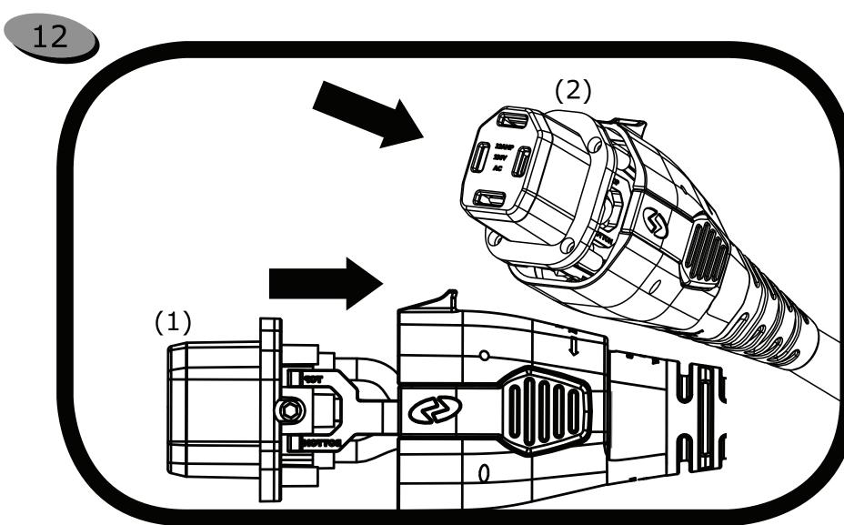
Hold cord seal and connector body in one hand as shown (1) and carefully pull cord with other hand backwards until it begins to enter connector body
