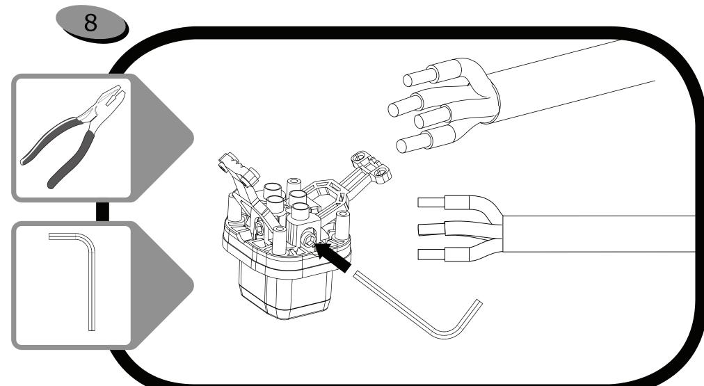
For ease of alignment, use pliers and slightly bend the ends of the conductor wires as shown. Next, use the provided hex key and loosen the set screws in the front connector assembly to allow plenty of clearance for the insertions of the copper strands into the inlet holes.
