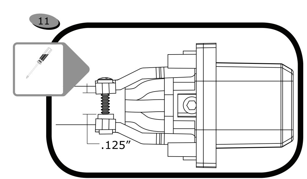
Use Phillips #2 screwdriver and tighten screws evenly about 1 turn each while alternating from one screw to the other until cable is sufficiently captured. Do not exceed 14lbs/in torque specification. Do not over tighten screws into cable clamp swing arm. A small gap as shown is acceptable, and should be even on both sides. About a 0.125" or 1/8" gap is correct. No gap may occur for smaller diameter cords.
