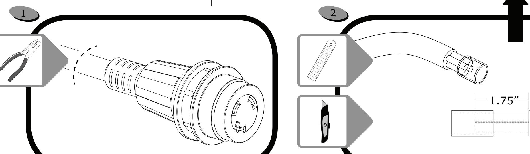
Cut female cord-end from your existing 50A 125/250V Cord-set. Inspect copper wires for corrosion, and cut back more cord if necessary to reach bright copper.
