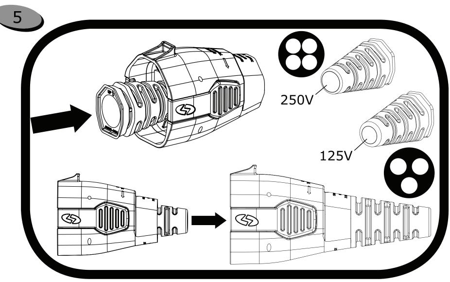
First determine appropriate cord seal for your particular cord diameter. Compress flexible cord seal and force into rear of plug body as shown. Align cord seal so grooved grip features are on the bottom and rotate cord seal until all 4 alignment ribs sin thir corresponding notches of the plug body. Look inside the plug body and inspect for proper cord seal fit. The seal should be fully expanded and free from folds or kinks. Set assembly aside.
