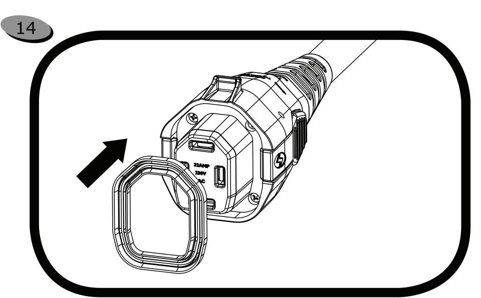
Remove adhesive backing from seal and slip over the plug face as shown. Use blunt tool and continue pushing seal into assembly until it seats and adheres fully. Check for any deformation of seal and adjust to fit.
