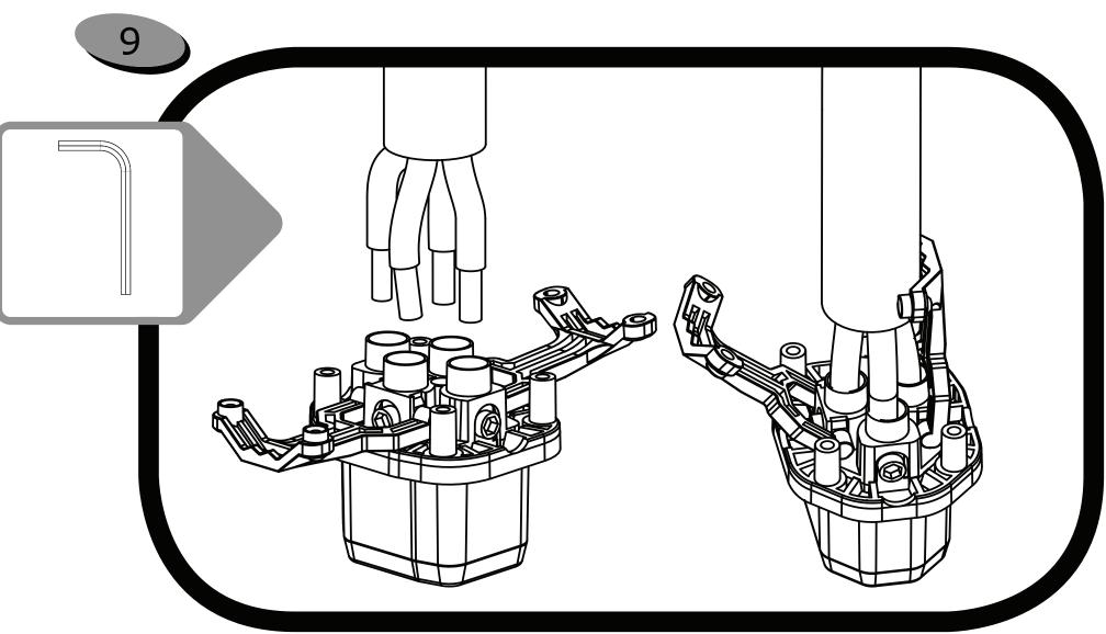
Simultaneously align and insert the individual wires into their corresponding color-coded inlets as shown. Push all wires in as far as they will go. Make sure all copper wiring is fully captured within the rear of the metal capture. Visually inspect through the clear plastic inlets that there are no stray copper strands. Use the hex key and tighten all screws to 20-25lbs/in
