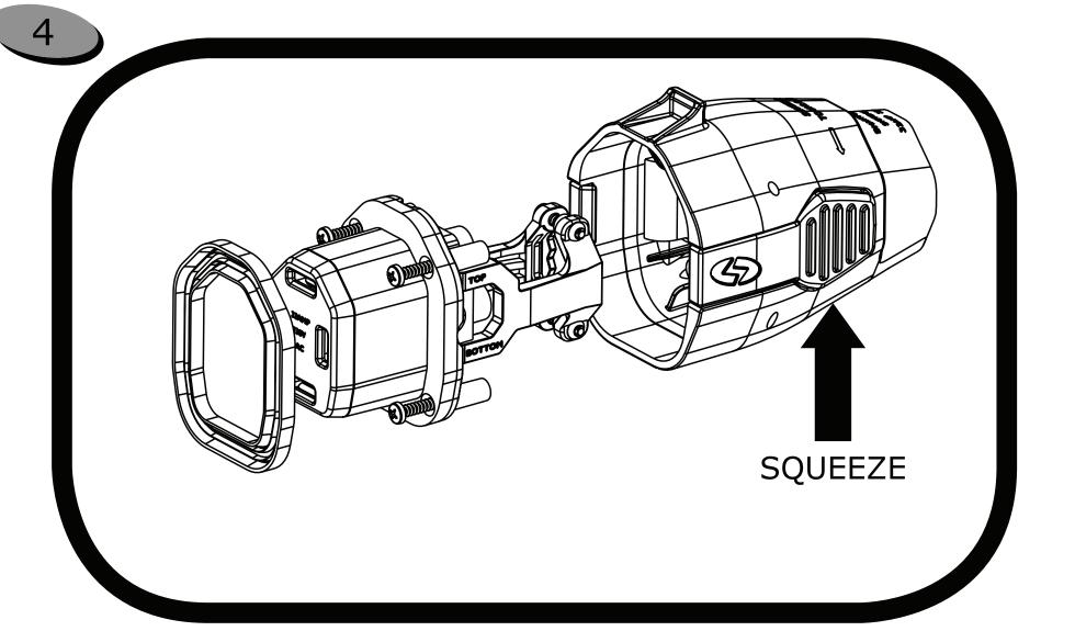
Separate the face seal, connector face and the 4 screws from each other by removing connector face from connector body. Squeeze levers and pull them apart. Set connector face assembly aside.
