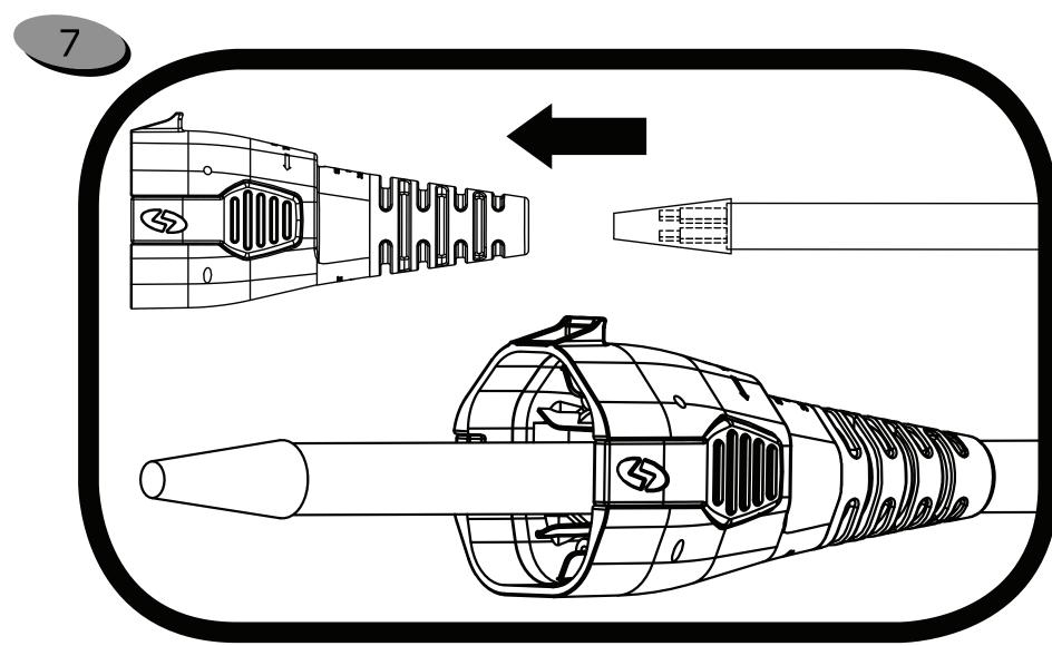
Push lubricated cord with cord install tool through cord seal and connector body from REAR as shown.
