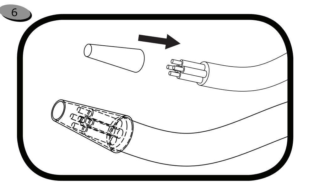
Use the cone shaped cord-install tool and cover the end of the prepared cord as shown. Apply liquid soap liberally on cord install tool and 12" of cord.
