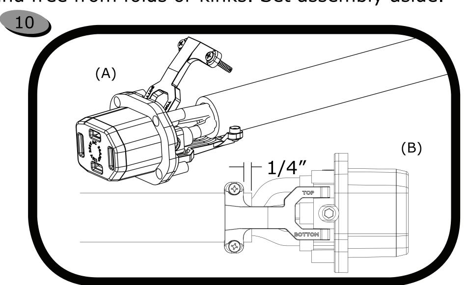
Close cable clamp arms around cable jacket as shown (A) and make sure a minimum of 1/4" of cable jacket extends beyond the jaws of the cable clamps (B). Insert (2) #6x1.25" screws (included) and pinch cable clamps around cable to hold them steady.
