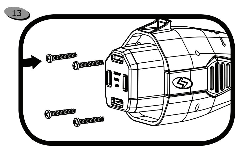
Locate and install (4) #6x1" screws (included) into corresponding inlet holes as shown. Use Philip's #2 and carefully screw components together by hand only.
