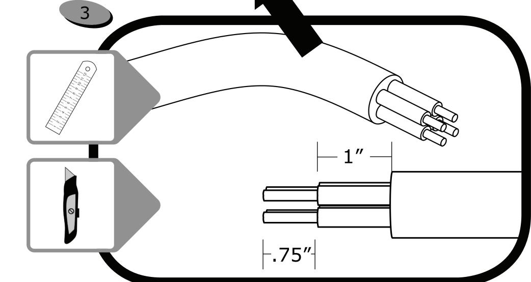
Measure and cut 0.75" of inner wire jacket from each of the individual color coded conductors.
