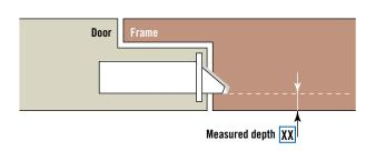
To find the right striker for your application, measure the distance from the door face to the edge of the springbolt of the latch.
